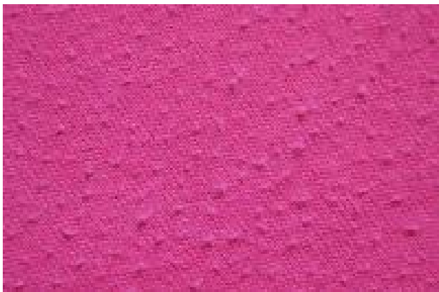
Fig. 8 Knitted fabrics with pilling made from yarns with high hairiness
