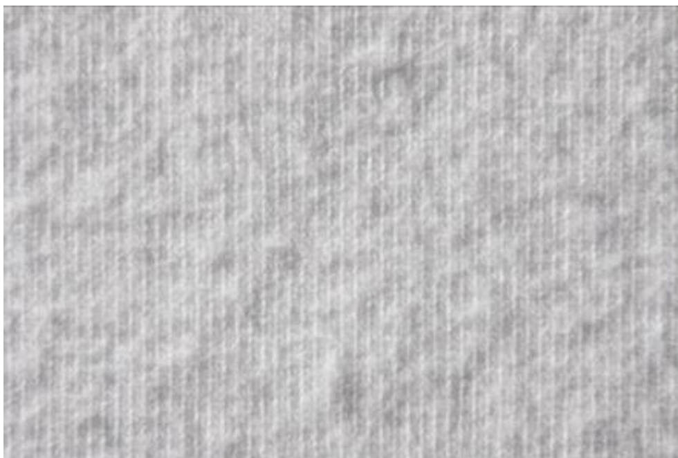
Fig. 33 Cotton yarn with high hairiness and pilling in a T-shirt
